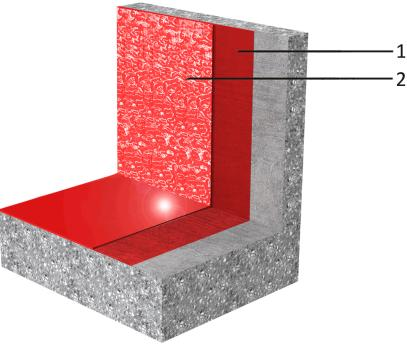
Sikafloor® MultiDur ET-39 V system (~1.5–2.0 mm)
