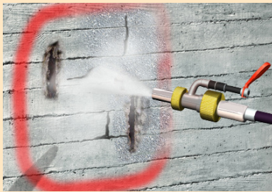
Removal of Damaged Concrete
