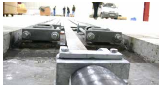
Base channel with post-tensioned CFRP plates
