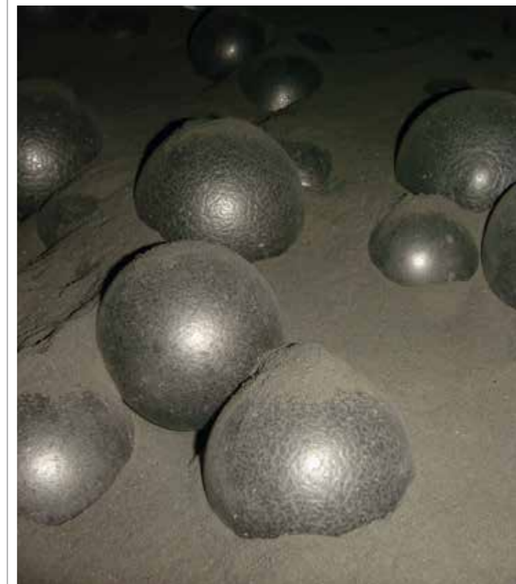
Grinding aids reduce the attraction of the fine particles and keep surfaces cleaner.
