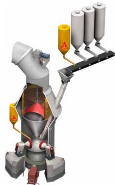
Vertical roller mill.
