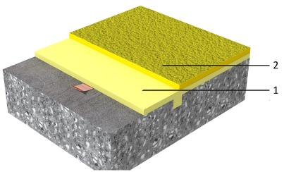
Earthing + Conductive scratch coat
