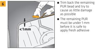
as possible ■ The remaining PUR must be under 1 mm
