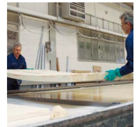
Positioning of the core foam
