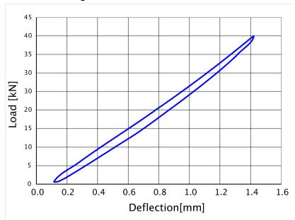
Static stiffness determined according to DIN 45673-1. Dimensions of test specimen 360  $\times$  160  $\times$  25 mm; Spring index  $k_{\text{stat}}$  = 29 kN/mm, determined as per the secant method between 8 and 32 kN.
